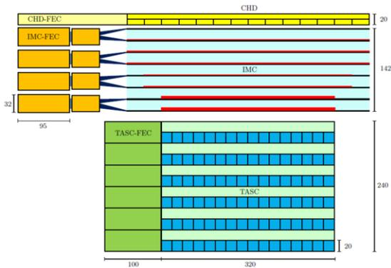
Figure 3: CALET instrument schematic side view. Dimensions are in mm.
