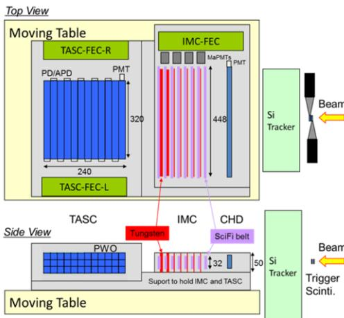
Figure 9: Configuration of the CALET prototype II for the beam test at CERN-SPS in 2011.
