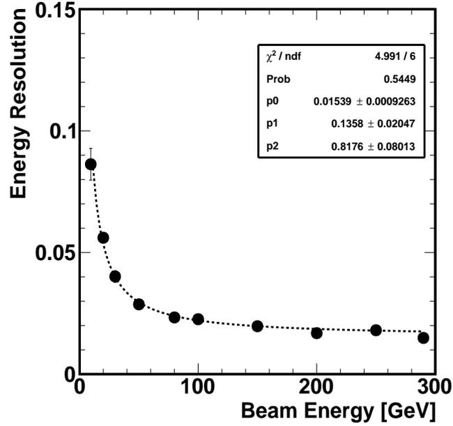
Figure 5: energy resolution for electrons from 10 to 290 GeV.
